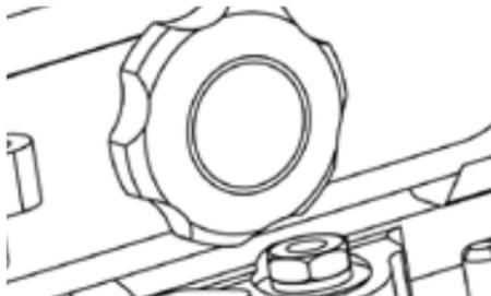
**Figure 2-1 Battery Compartment Knob**
