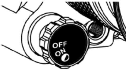
**Figure 3-8 Polarity Momentary Switch**
